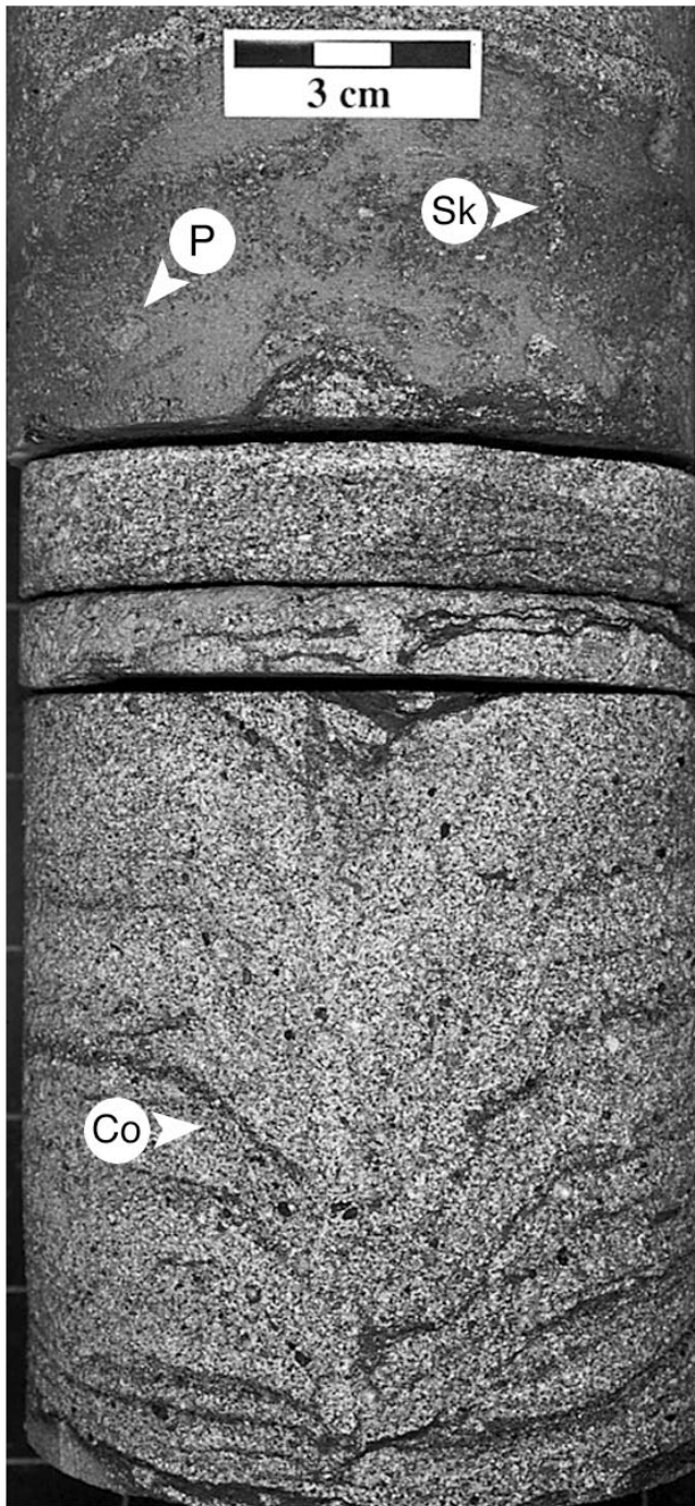
Figure 13—Core showing facies A, which is a highly glauconitic, trough cross-stratified sandstone overlying BD-2. A robust Conicbnus (Co) is present within the sandstone. Siderite-cemented zone toward the top of the photo contains Planolites (P) and Skolithos (Sk). This facies is interpreted to reflect transgressive sand sheets mantling BD-2 within the embayment (well 01-07-38-24W4, 1416.0 m).
