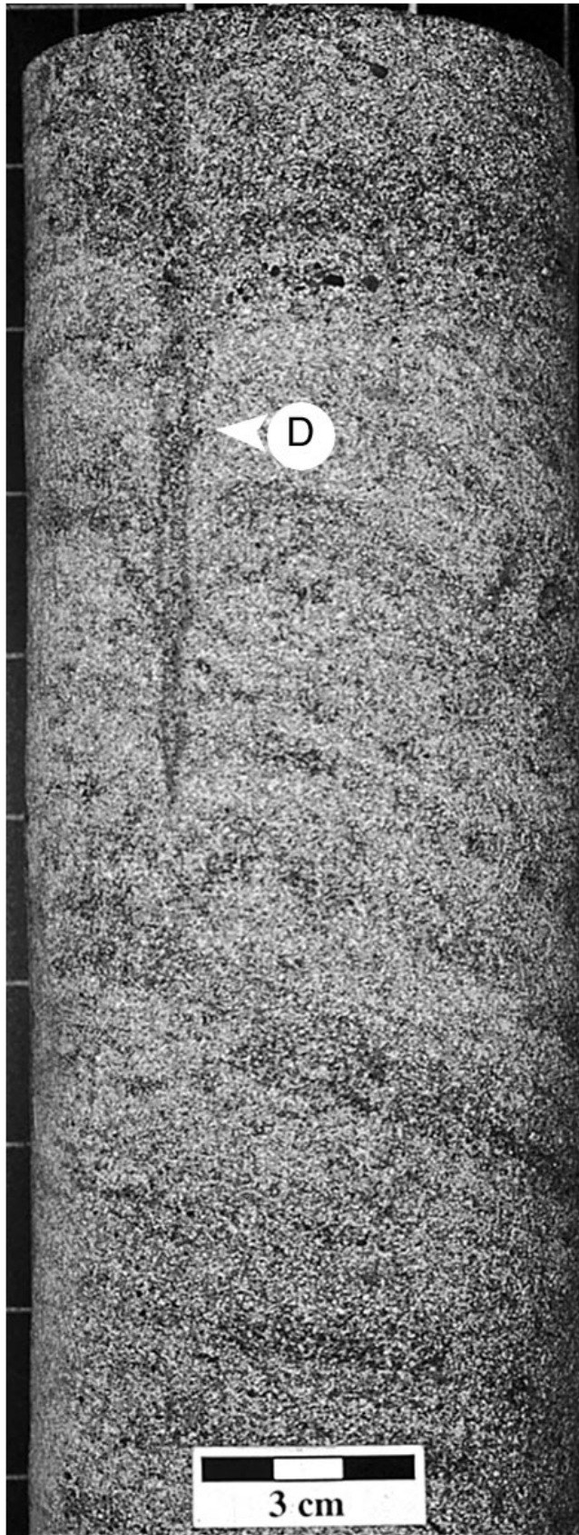
Figure 14—Core showing facies B, a large-scale trough cross-stratified sandstone with a lined Diplocraterion (D) shaft. This facies is interpreted to reflect migrating dunes within marginal marine (brackish water) channels (well 02-05-39-26W4, 1573.3 m).
