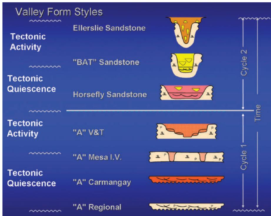
FIG. 40.—Variations in BQ valley form and width:depth ratios. Cycles 1 and 2 relate to tectonic stages of the adjacent Cordillera during accumulation of the Basal Quartz (as defined in Zaitlin et al., 2002). Note how in each cycle the first valleys are broad and relatively shallow, whereas younger valleys have greater depth-to-width ratios.
