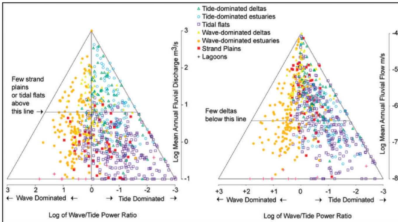
FIG. 53.—Coastal classification and empirical model testing from Harris et al. (2002). In this approach, the parameters of log [mean annual fluvial flow] (vertical axis, right) and fluvial discharge (left) have been plotted on a ternary diagram against log [ratio of tidal power to wave power]. This provides a quantitative test for the Boyd et al. (1992) coastal-classification scheme using all the river mouths on the Australian coast. Note segregation of major coastal depositional settings.
