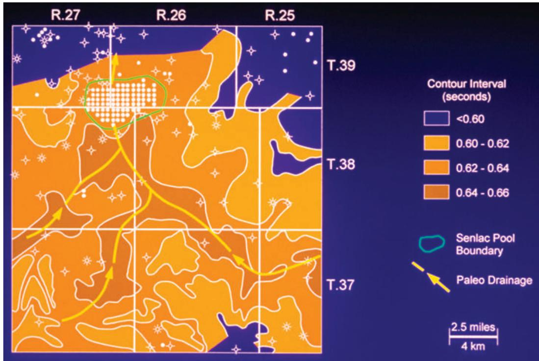
FIG. 35.—Two-way travel time in seconds to the sub-Cretaceous unconformity in the Senlac area of southwestern Saskatchewan, Canada. Darker colors (longer times) indicate areas where the unconformity is deeper. The pattern is interpreted to represent an incised-valley network. Arrows indicate interpreted paleovalley trends and inferred paleodrainage directions. (From Zaitlin and Shultz, 1990.)
