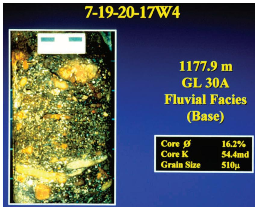
FIG. 30.—A typical basal pebbly fluvial-lag facies from the Lathom “A” 7-19-20-17W4 well, with its associated grain size, porosity ( $\emptyset$ ), and permeability (K) values (from Zaitlin et al., 1998).
