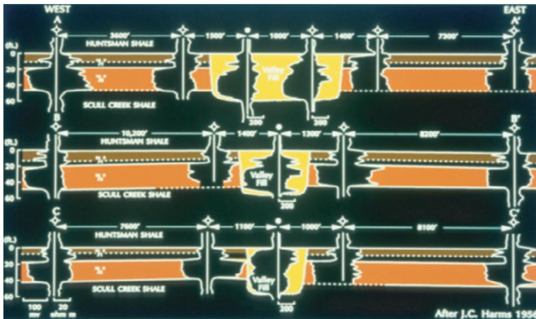
FIG. 2.—Wireline-log cross section from Harms (1966) showing one of the first and best-described examples of a subsurface depositional system meeting the criteria of an incised valley—the Cretaceous “J” Sandstone in western Nebraska. The figure shows the J Sandstone as “valley fill”, incising the regional Skull Creek Shale and Huntsman Shale.
