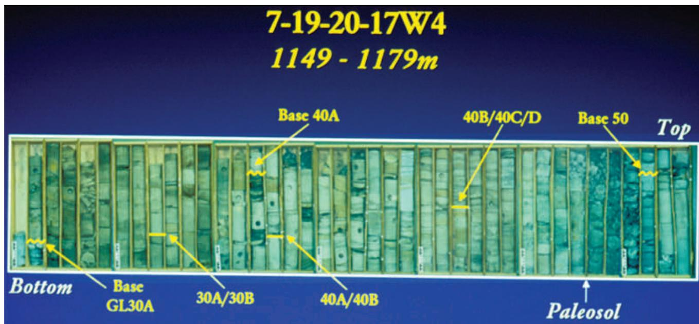
FIG. 28.—An example of a compound incised-valley fill from the type Lower Cretaceous Glauconitic Formation well from the Latham “A” field in southern Alberta, Canada. (Zaitlin et al., 1998). Bottom of core to the lower left; top to the top right. Glauconitic Sandstone Member; 30, 40, and 50 represent informal units in the Glauconitic; A = fluvial facies, B = tidal–fluvial, C/D = tidal–fluvial bayhead-delta to central-basin facies.
