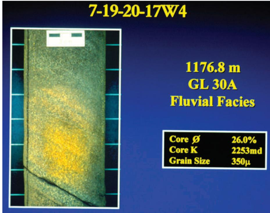
FIG. 31.—Sandy cross-bedded fluvial facies from the Lathom “A” 7-19-20-17W4 well, with its associated grain size, porosity ( $\emptyset$ ), and permeability (K) values (Zaitlin et al., 1998).
