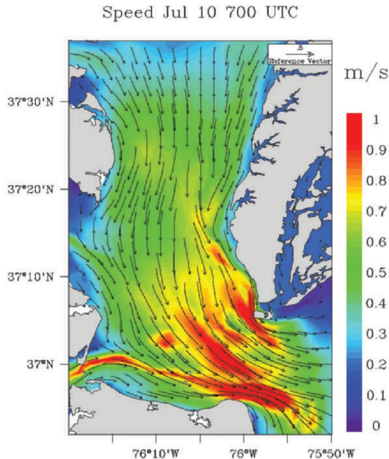
FIG.52.—Animation of tidal circulation in Chesapeake Bay. (From <http://ccmp.chesapeake.org/C3POANIM/>). Color bar on right shows surface tidal current speed in m/s at 0700 on July 10, 2006. Arrows on figure show direction of water transport.
