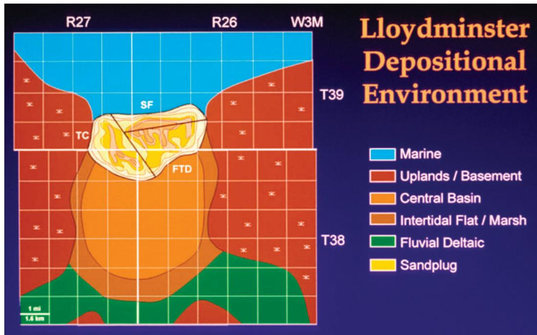
FIG. 36.—Distribution of inferred depositional environments during Lloydminster Formation time in the Senlac incised valley. SF. = shoreface deposits; TC. = tidal-channel deposits; FTD = flood-tidal-delta deposits. Heavy black lines separate depositional environments within the estuary-mouth sand plug. (From Zaitlin and Shultz, 1990.)
