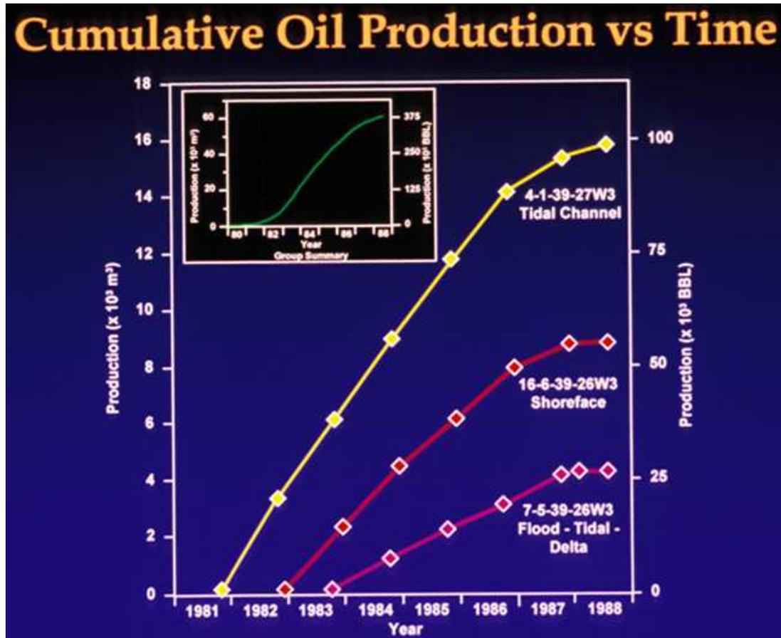
FIG. 38.—Plot of cumulative oil production vs. time for three typical wells completed in the tidal-channel, shoreface and tidal-delta lithofacies. Inset: total cumulative oil production vs. time for the Senlac Pool. (From Zaitlin and Shultz, 1990.)
