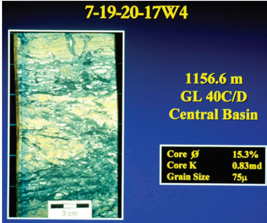
FIG. 34.—An example of bioturbated central-basin facies from the Lathom “A” 7-19-20-17W4 cored well, with its associated grain size, porosity ( $\emptyset$ ), and permeability (K) values (from Zaitlin et al., 1998).
