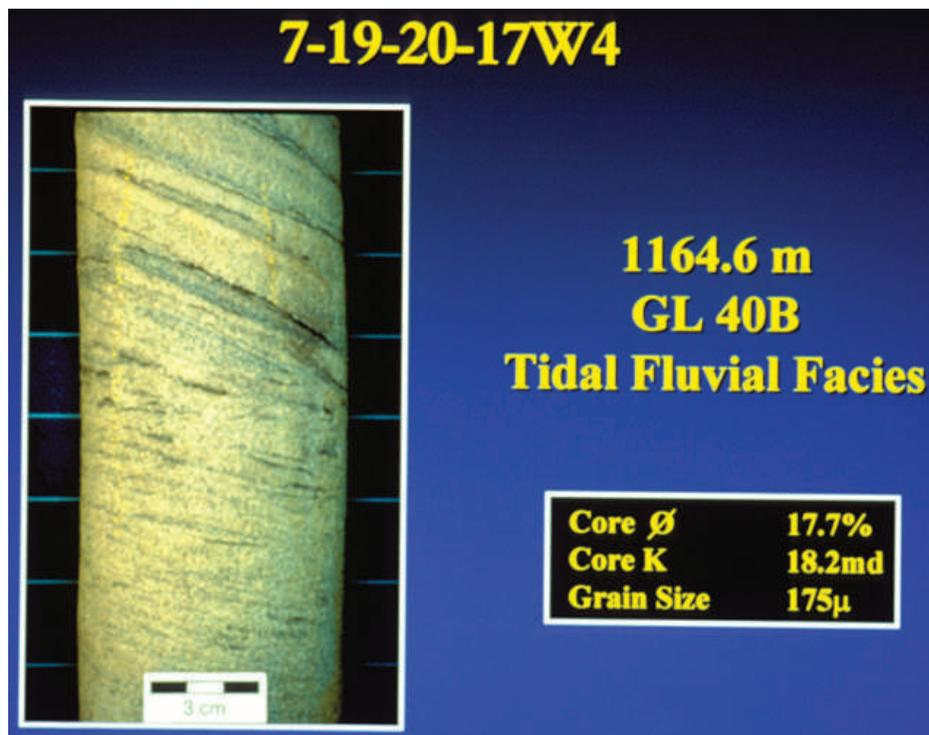
FIG. 32.—Typical tidal-fluvial facies with tidal couplets and mud drapes from the Lathom “A” 7-19-20-17W4 cored well, with its associated grain size, porosity ( $\emptyset$ ), and permeability (K) values (from Zaitlin et al., 1998). The mud layers reduce permeability and make this facies a poorer reservoir than the fluvial facies (Figs. 30, 31) that underlie these deposits (see Fig. 29).
