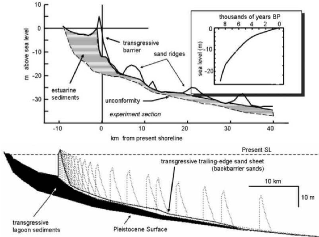
FIG. 50.—Transgressive shoreface simulation of Duck, North Carolina, U.S.A., showing retention of a thin estuarine valley fill (horizontal stripes) after shoreface translation during the last 9 ky (sea-level curve in upper right). From Cowell et al. (1999) and Cowell et al. (2003).
