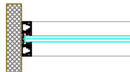
Exposed wall abutment for single middle glass application
