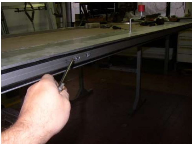
1 - Unscrew and remove the mobile head profile
