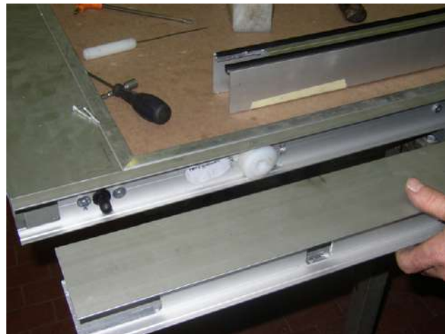
5 - Extract WITH CARE the whole gear shaft (push FROM bottom TO top to let slide it)
