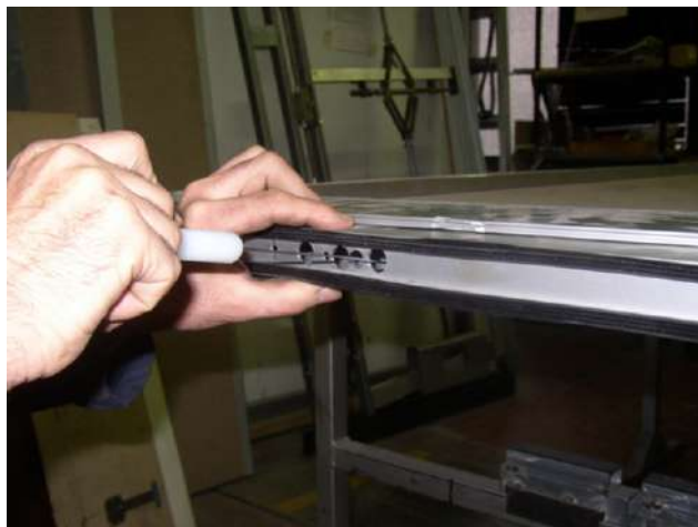
2 - Unhook mobile seal springs
