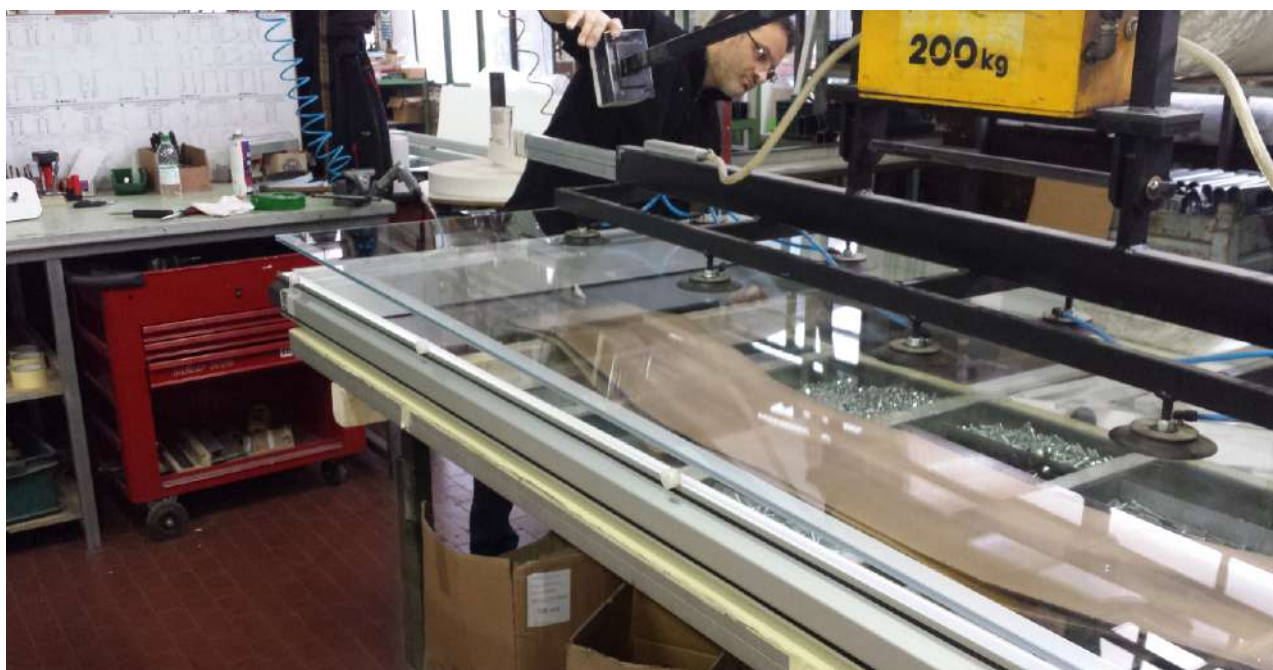
PHASE 2: GLASS FIXATION GUIDED BY SPACERS
