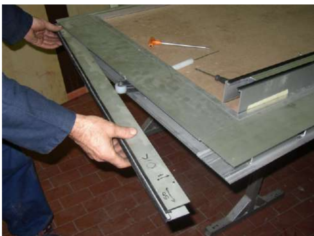
3 - Partially extract (NOT fully) mobile seals as shown
