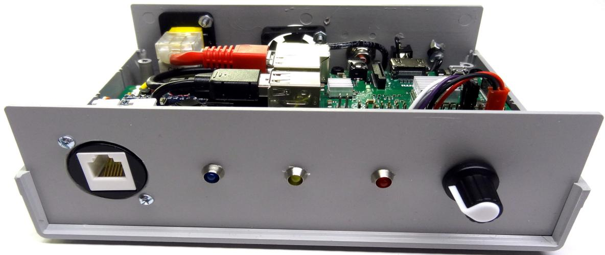
*Front panel showing the RJ11 microphone connector, PTT (blue), COS (yellow), and power (red) indicators and the volume control.*
