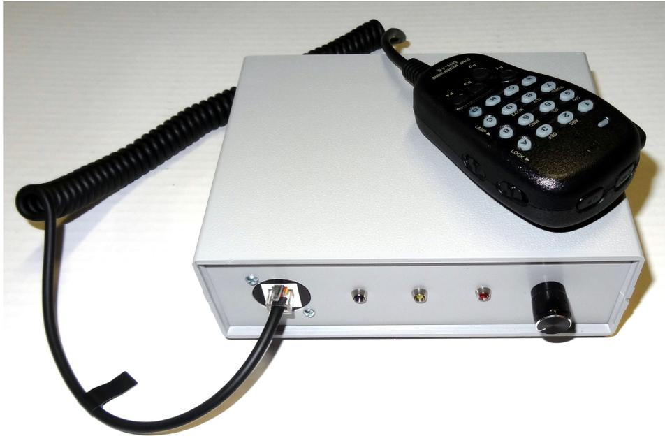
The ARN-1 radio-less node allows direct wired or wireless Internet connection to the Amateur Radio Allstar network as well as Echolink, IRLP, and other digital modes. It is an all in one communications solution for fixed or mobile locations. Some of the features include -
