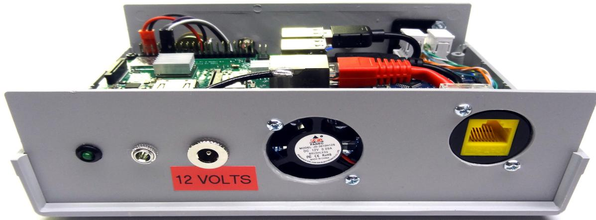
*Rear panel showing heartbeat (green) LED, miniature Speaker Jack, 12V power input, cooling fan, and Ethernet connection.*
