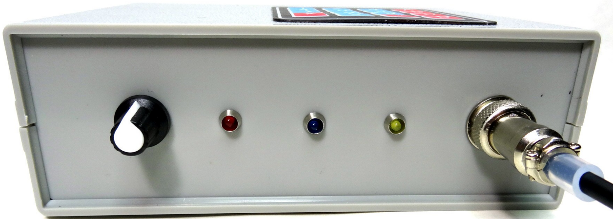
Front panel showing the Volume control, power (red), PTT (blue), COS (yellow) LED indicators and the 8 pin round microphone connector.
