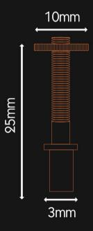
A speficially designed fitting that can be custom built onto EndGlow fibre arraying in different sizes. However, it can also be sold seperately to fix onto pre-existing fibre.
