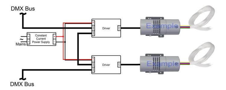
LFM can be connected only with serial wiring. LFM may be connected to driver. Above connection is examples and may be different from the actual.
