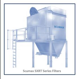
Scumax SXRT cassette type dust collector (reverse air impulse cleaning) includes an inlet hood for dust-crude gas, the filter casing and the dust collection hopper with support structure and a discharge unit.
