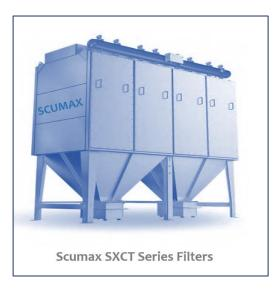
Scumax SXCT Cartridge type dust collector, the construction of this filter cartridge elements in a cartridge filter system are built out of fine filter media arranged in a pleated manner, due to which a very large filter area is accommodated in a very small cylindrical shape. The net effect is that a cartridge filter system occupies much smaller area and space compared to a conventional bag filter system (one-eighth).
