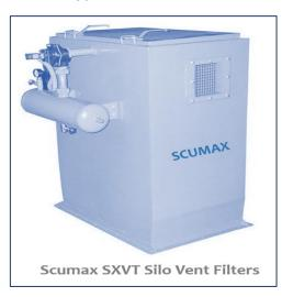
Scumax SXVT silo vent filters, a compressed air cleaned cartridge filter with 87m2 filter surface, used for silo ventilation. Also available with 3.7 hp fan assist, strong welded construction. Filters can be replaced very easily as hinged lid opens upwards and the cartridge are replaced from above needless to say.
