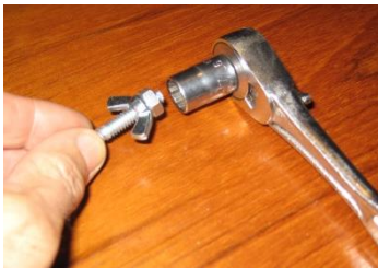
Use Jam Nut to Drive in Hanger Bolts
