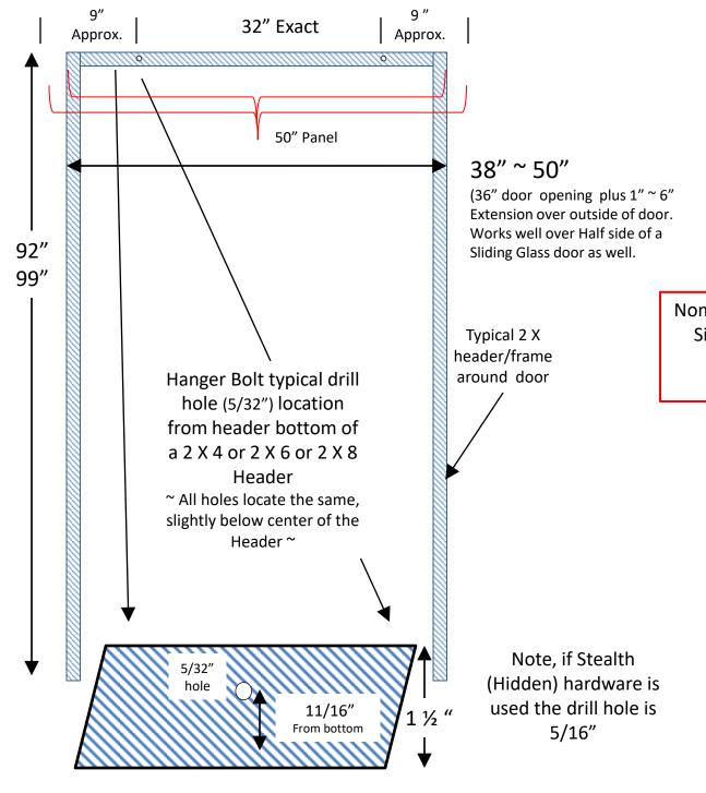
Nominal 3-4 Foot (36"-48") Wide, 8 Foot (96")Tall Single Door or Half Side of Sliding Glass Door Guideline Drill distance locations for PARTAYGARAGE Hanger Bolt hardware.
