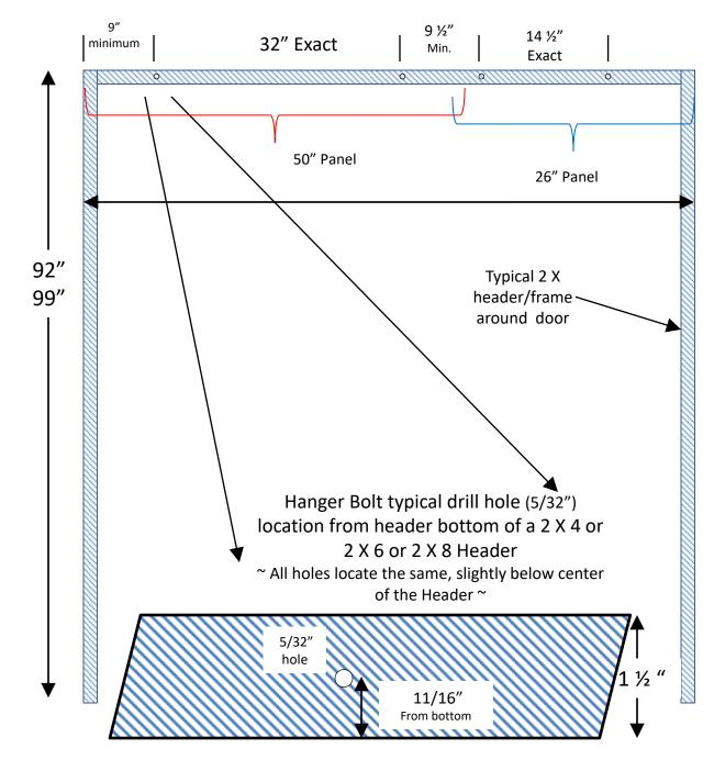
Note, if Stealth (Hidden) hardware is used the drill hole is 5/16"
