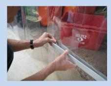
2. Locate and push the two outboard studs of the Weight thru the pair of pre-perforated holes in two outer slats of a 50" PARTAY Panel, both sides respectfully. Make sure that the slats stay in their front/back/front/back respective positions. Loosely secure wing nuts on both of the outer studs.
