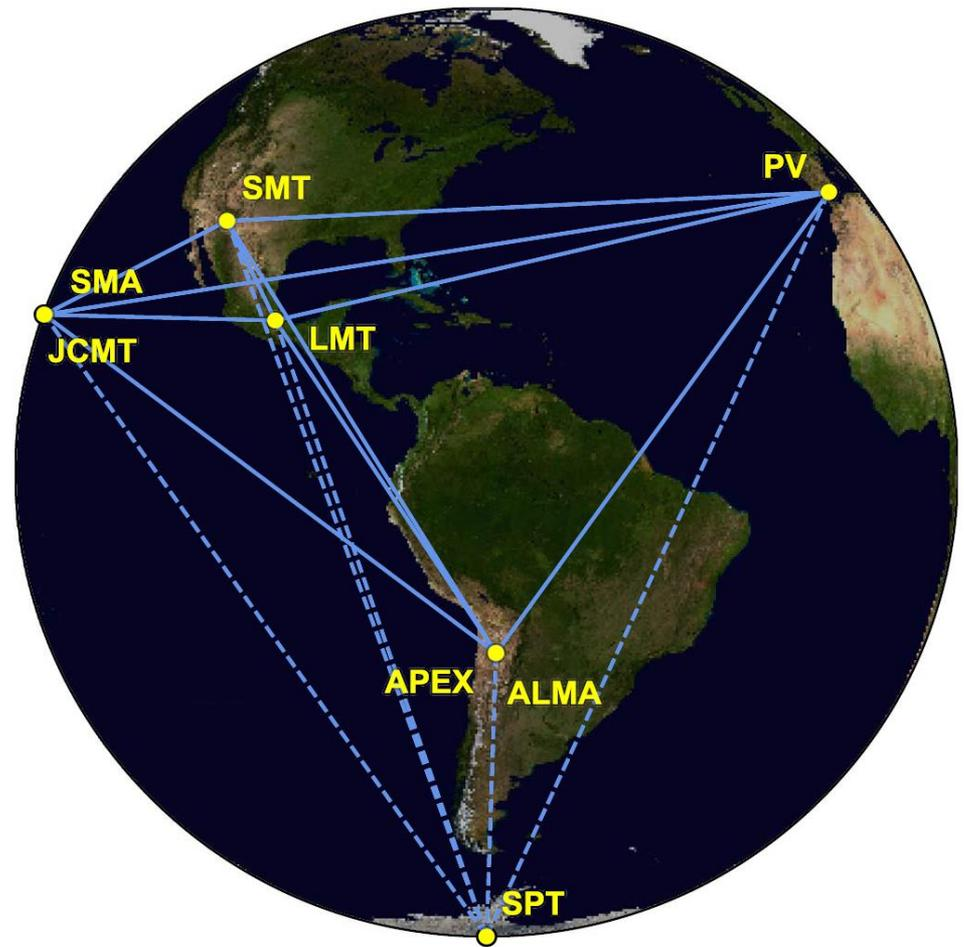
**Figure 1.** Eight stations of the EHT 2017 campaign over six geographic locations as viewed from the equatorial plane. Solid baselines represent mutual visibility on M87\* (+12° declination). The dashed baselines were used for the calibration source 3C279 (see Papers III and IV).
