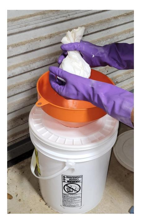
21\_(6:30 pm) Wrung out (polymeric) solids wearing heavy duty rubber gloves (this filter paper is doubled commercial coffee/tea filter paper (originally 24" diameter cut to size for this application)
