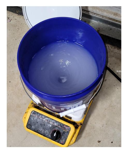
30\_To blue bucket containing washed hexane layer (below) was added brine (1 Kg). Mixture stirred 10 min (right) then transferred to separatory funnel and separated
