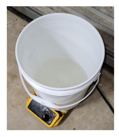
26\_Drained (lower) aqueous layer back into (white) 5 gallon bucket. Drained (upper) hexane layer into (blue) 2 gallon bucket containing first extract
