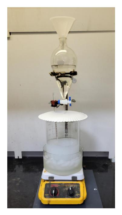
5\_(12:05 pm, IT = 17) Filled crystallizing dish halfway with water
