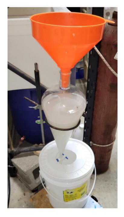
24\_Added 800 g hexanes (2<sup>nd</sup> extraction) to aqueous layer and stirred 10 min (below)
