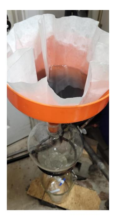
15\_ Layers were separated and to the (top) 2-MeTHF (organic) layer (in a 4 L beaker containing a 3" stir bar) was added 300 g DI water. After stirring vigorously, poured back into sep funnel. [Note this aqueous wash was unnecessary (skip next time) as separation of layers was slow (EMULSION)]. Let sit in sep funnel 20 h after which time the emulsion completely broke.
