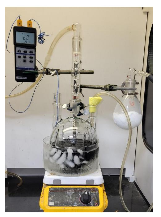
10\_ Let RM stir at RT ~1.5 h and then cooled to 5 °C. Began bubbling in CO<sub>2</sub> (from a 500 mL RB flask loaded with 200 g dry ice) through Tygon tubing and a glass pipet (see photo- Left)
