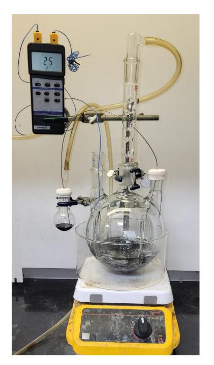
7\_ A 500 mL addition funnel was incorporated and charged with a solution of piperonyl chloride (328 g) in 2-MeTHF (150 g)- see photo- Right.
