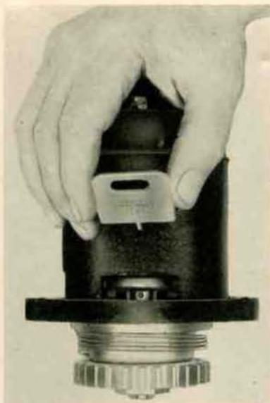
**Fig. 2. Timing Hole and Gage**
