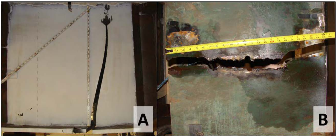
Figure 6.32: Fracture Test 2 fractured main girder web (A) & bottom flange (B)
