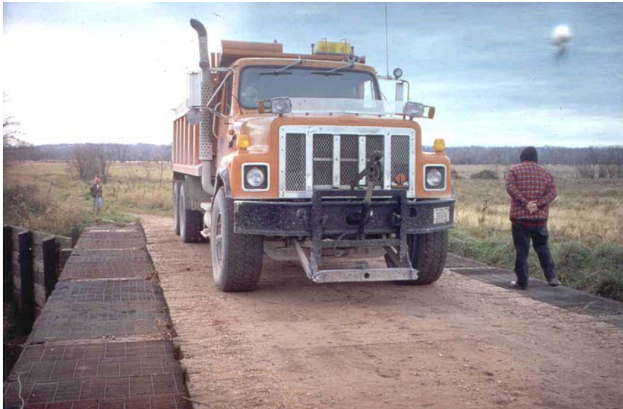
Figure 4.6. Photograph of rear tandem-axle test truck in position C2.
