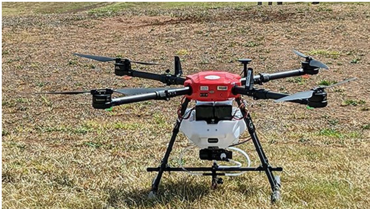
Fig. 7. Drone used for foliar application (Source: UH Press, 2022 ).
