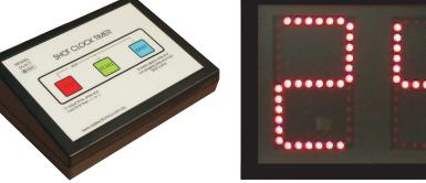
When a shot is in progress, press and hold down the RESET button. This will blank the shot clock displays and will reset the timer. When the RESET button is released the shot clocks will start counting down from the SET time ( Default 24 seconds)
