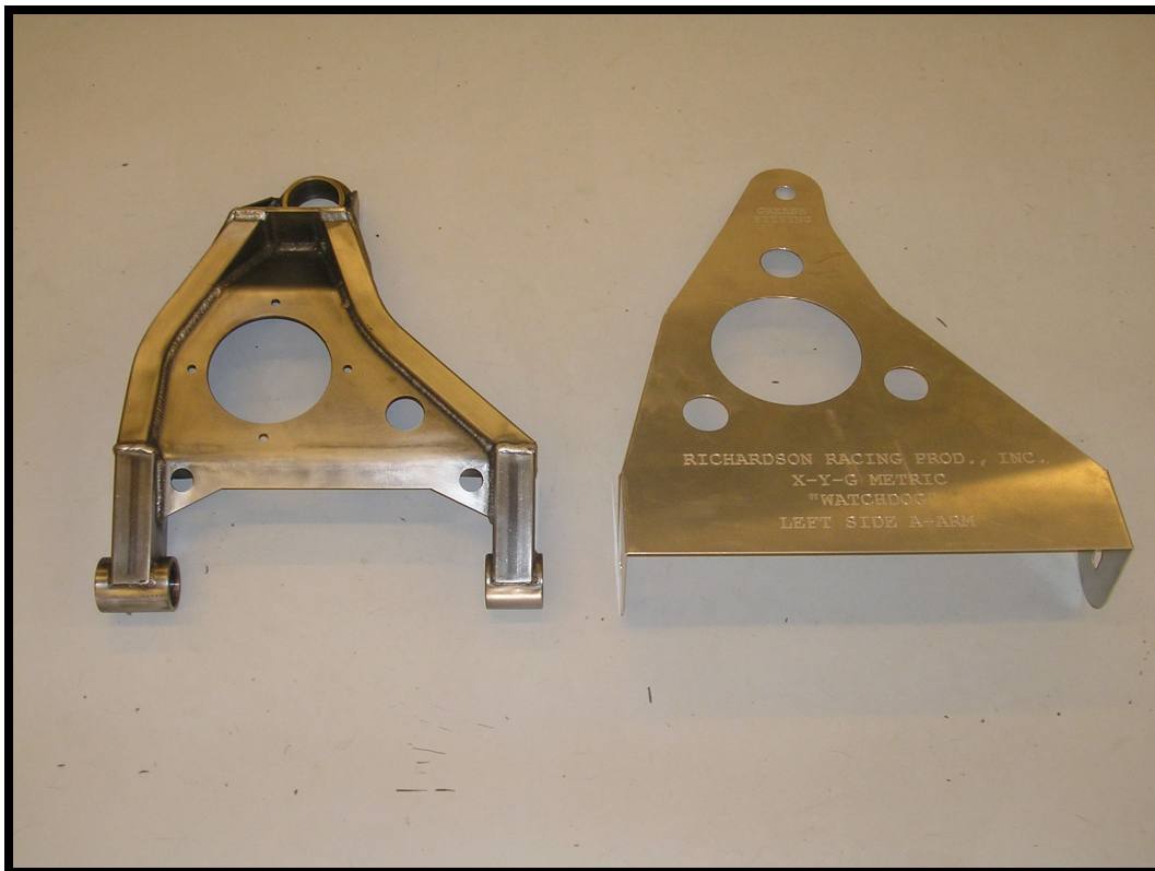
INSPECT A-ARMS ON THE CAR NO-GO
