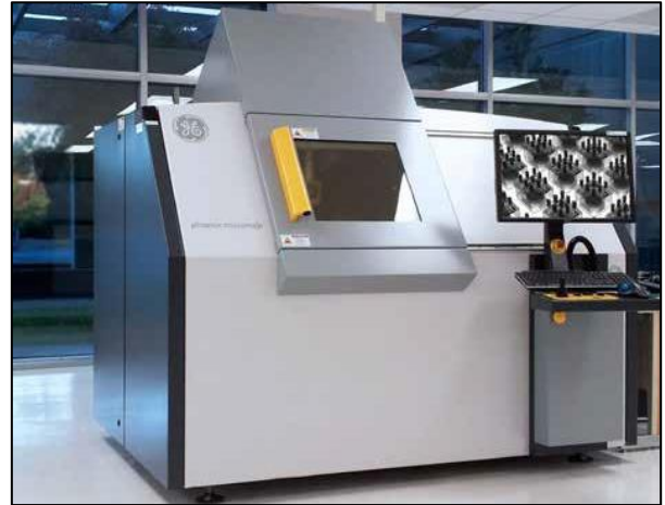
Figure 1 – Axiom uses x-ray inspection to set up processes and inspect mission critical products.
