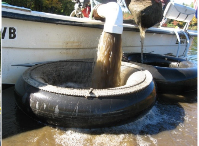
“Dash” boat pushing water and milfoil through strainer near Kezar Falls Dam
