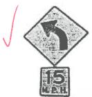
Post physical warning signage (yellow with black lettering) that recommends reduced speeds at specific sharp curves and dangerous intersections.
