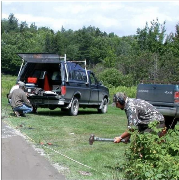
Operating a twelve-channel seismograph, Piscataquis County, Maine.
