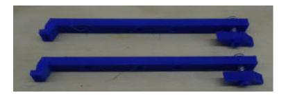
Using the two mounts and two M3×8MM screws, attach mounts as shown. The off-set nuts will be at the bottom. Hand tighten the screws only!
