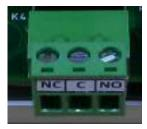
This relay output is rated at 120VDC at 5 amps. Used to disable automatic door control(s).
