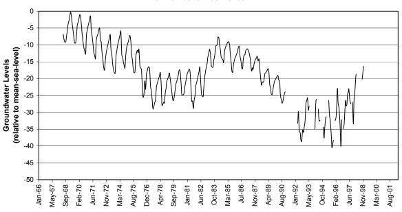
Groundwater Levels for Observation Well #1 Well Number 07N06E23P001M
