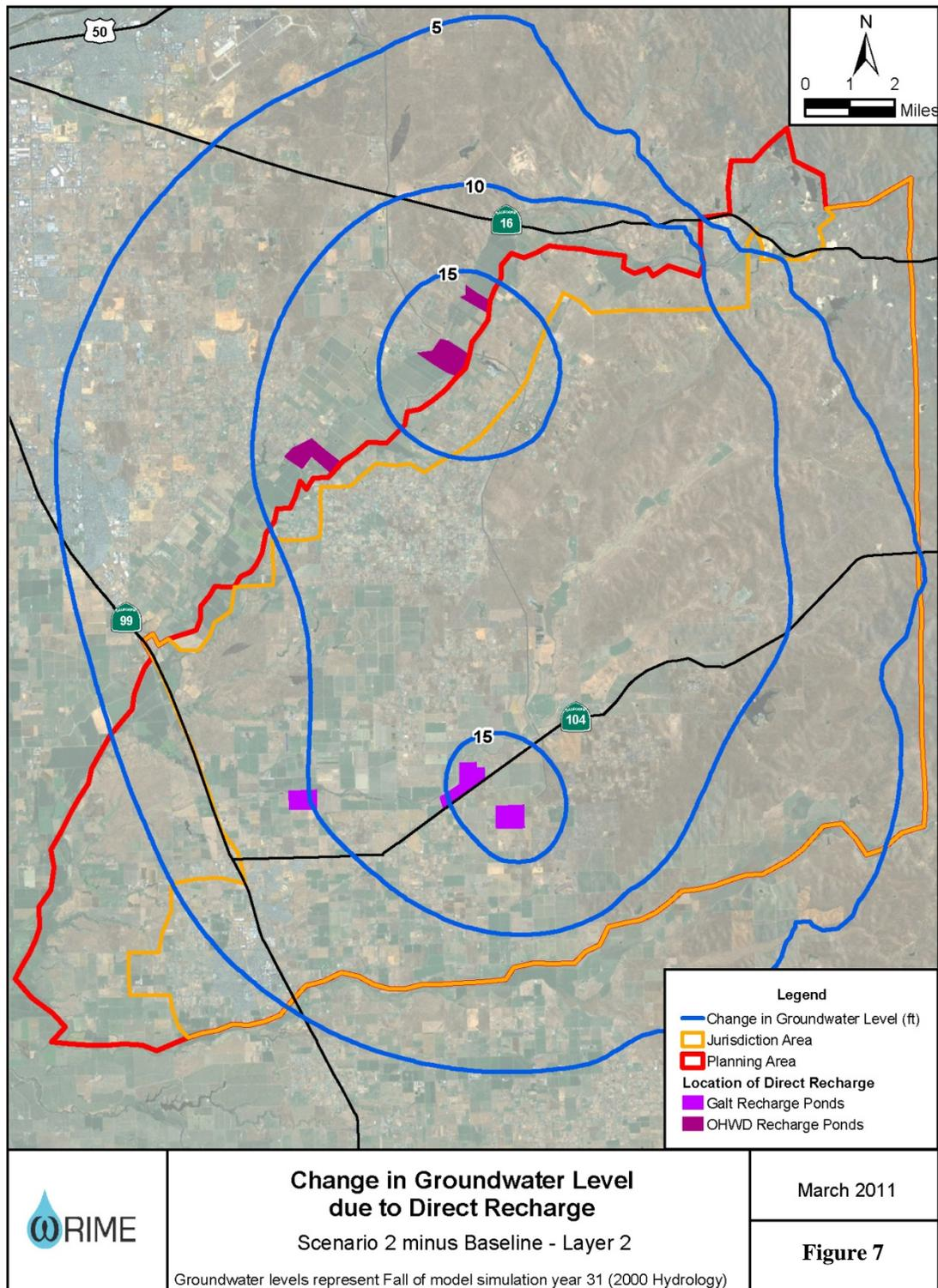
Figure 5-7. Change in groundwater level due to Direct Recharge – Layer 2.
