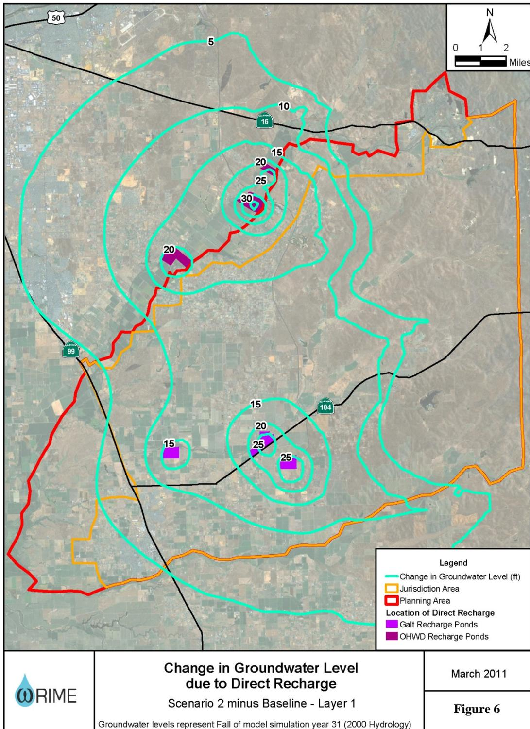
Figure 5-6. Change in groundwater level due to Direct Recharge – Layer 1.
