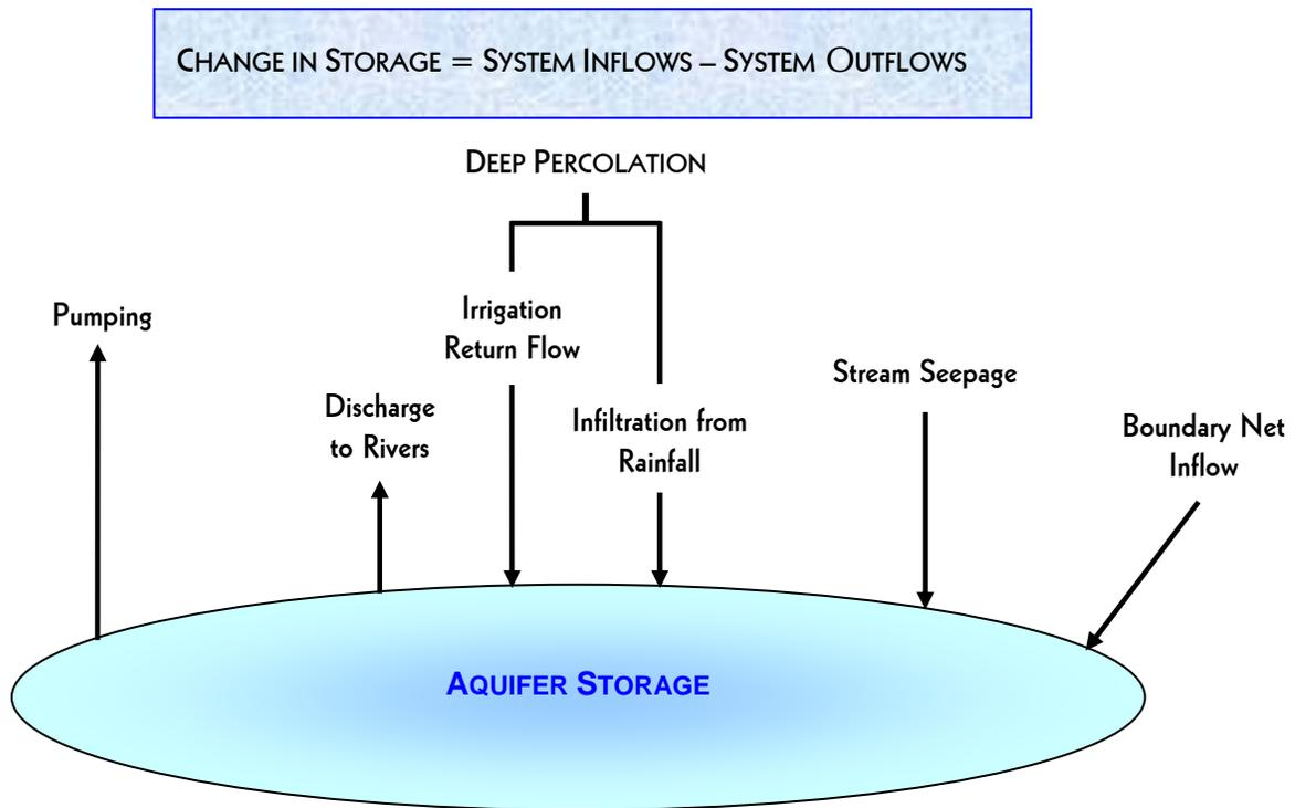
Figure 1-22. Groundwater balance components, South Basin.
