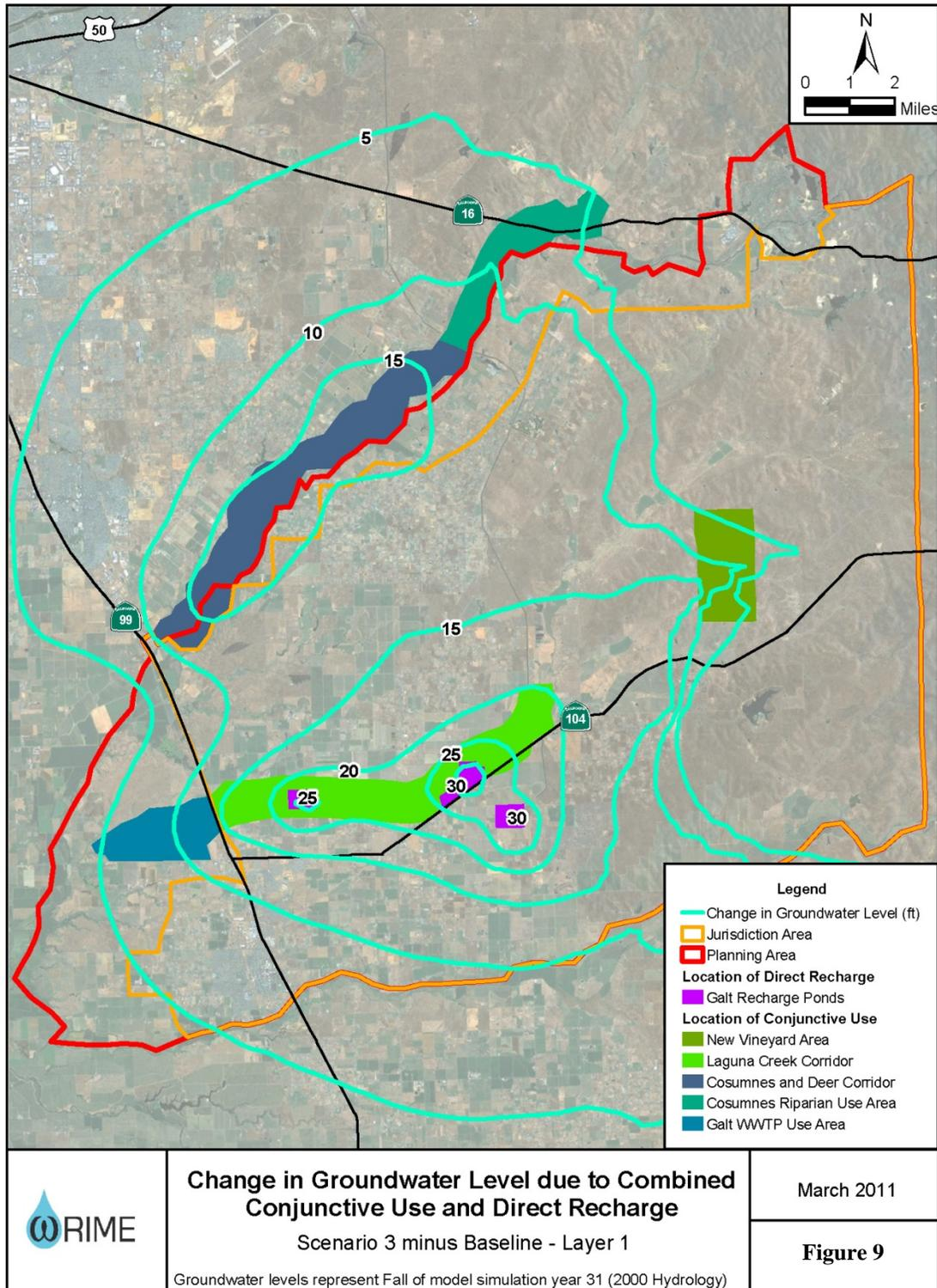
Figure 5-9. Change in groundwater level due to Combined Conjunctive Use and Direct Recharge – Layer 1.
