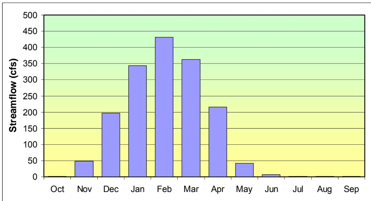
Figure 1-9. Average monthly streamflow on Dry Creek near Galt for 1926 to 1997 (USGS data).
