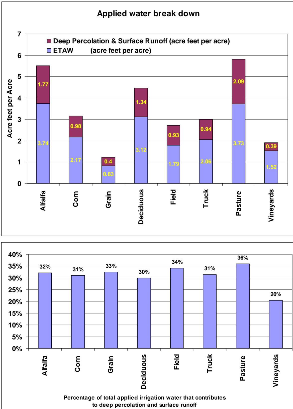
Figure 2. Applied water breakdown and percentage of total applied irrigation water that contributes to deep percolation and surface runoff, DWR Water Use Survey.
