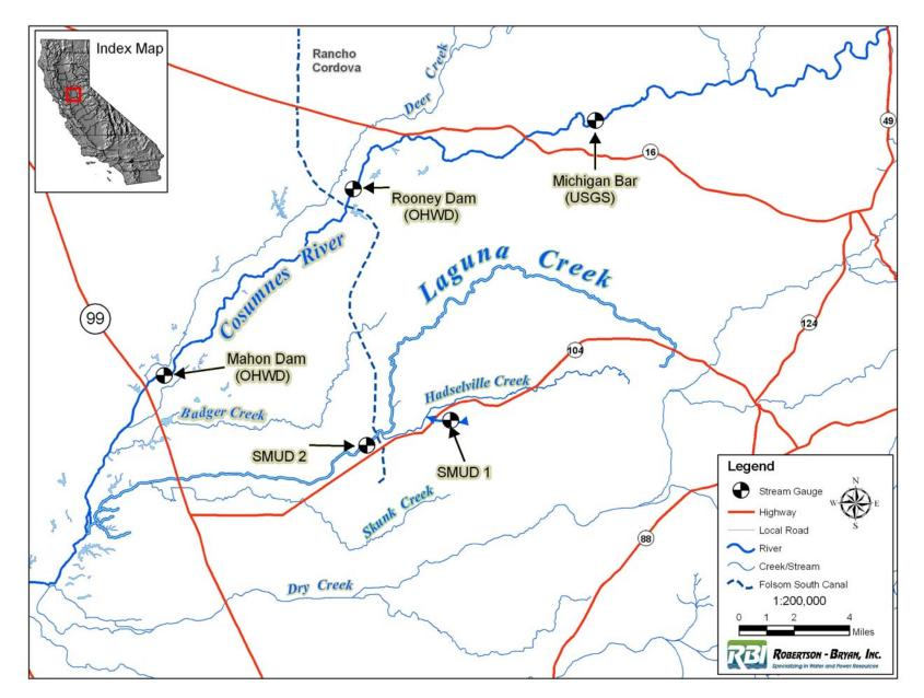
Figure 3-3. Location of stream flow gauges.
