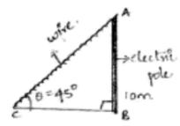
Height of the electric pole H = 10m = AB angle made by steel wire with ground (horizontal)  $\theta = 45^{\circ}$
