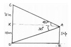
Height of ship from water level = 10cm = ABAngle of elevation of top of cliff  $\alpha = 45^{\circ}$ Angle of depression of bottom of cliff  $\alpha = 30^{\circ}$ Height of cliff CD = h'm. Distance of ship from foot of tower cliff Height of cliff above ship be 'a'm Then height of cliff = DX + XC=(10+0)m
