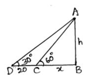
Let AB be the T.V tower of height 'h'm on a bank of river and 'D' be the point on the opposite of the river. An angle of elevation at top of tower is 60° and form the point 20m away them angle of elevation of tower at the same point is 30°
