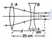
As the incident ray is parallel to the principal axis. Therefore in absence of concave lens it will form an image at focus of convex lens.
