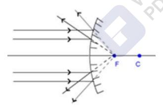
Answer: Convex mirror has a larger field of view because it is diverging in nature. The light rays incident on it gets diverged following the laws of reflection, the reflected rays form the wider path as shown in the figure below. illected ray
