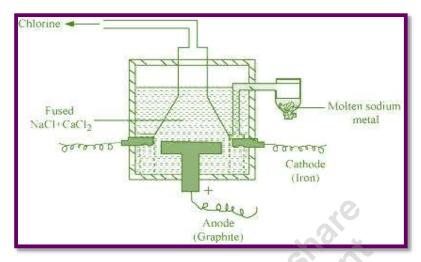
Steel is the cathode and a block of graphite acts as the anode. Metallic Na and Ca are formed at cathode. Molten sodium is taken out of the cell and collected over kerosene.
