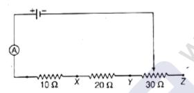
**Answer:** The current when it is connected to x is 0.6 A, so net resistance is 10 ohms so the cell voltage is  $10 \times 0.6 = 6 \text{ V}$ .
