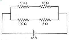
Answer: Here, the resistances  $10\Omega$  and  $15\Omega$  are connected in series and also the resistances  $20\Omega$  and  $5\Omega$  are also connected in series.
