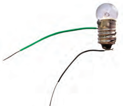
Fig.12.4 Bulb connected to two wires
