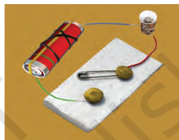
Fig 12.9 An electric circuit with a switch
