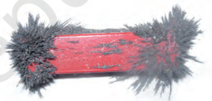
Fig. 13.7 Iron filings sticking to a bar magnet
