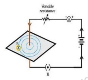
Right hand thumb rule states that if a current carrying straight conductor is supposedly held in the right hand with the thumb pointing towards the direction of current, then the fingers will wrap around the conductor in the direction of the field lines of the magnetic field.
