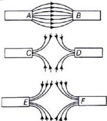
**Answer: (i)** A is North Pole and B is South Pole because magnetic field lines originate from North Pole and ends at South Pole.
