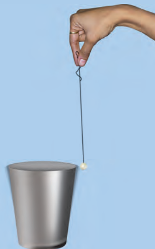
Fig. 13.17 : Thermocol ball touching the vibrating glass tumbler
