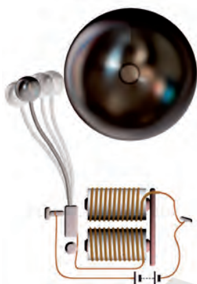
Fig. 14.20 Circuit of an electric bell
