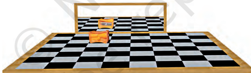
Fig. 15.7 Locating image in a plane mirror
