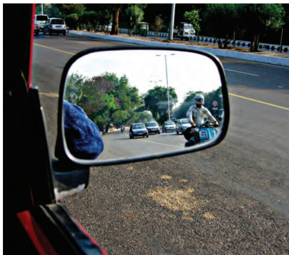
Fig. 15.20 Convex mirror as side view mirror
