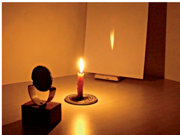
Fig. 15.15 Real images formed by a concave mirror
