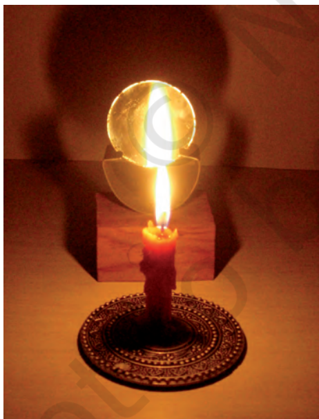
Fig. 15.16 Virtual image formed by a concave mirror
