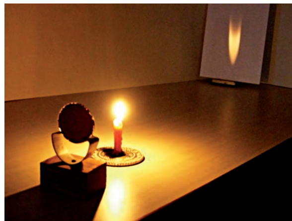
Fig. 15.15 Real images formed by a concave mirror
