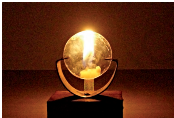
Fig. 15.26 Virtual image formed by the convex lens
