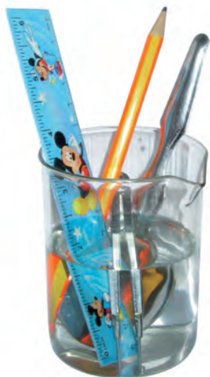
Fig. 4.8 Conduction of heat by different materials
