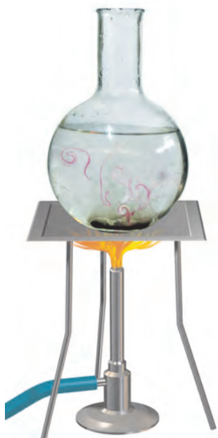
Fig. 4.9 Convection of heat in water
