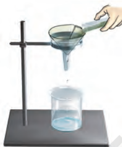
Fig. 5.10 Filtration using a filter paper
