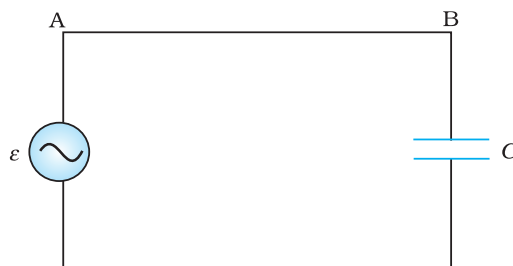
FIGURE 7.8 An ac source connected to a capacitor.
