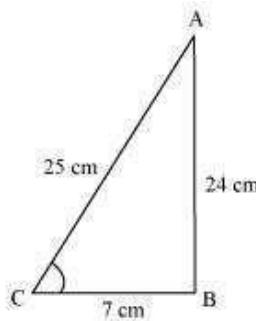
$$\sin C = \frac{\text{Side opposite to } \angle C}{\text{Hypotenuse}} = \frac{AB}{AC} = \frac{24}{25}$$
