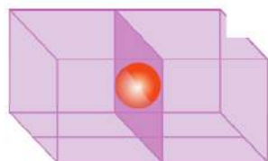
Fig. 1.15: An atom at face centre of unit cell is shared between 2 unit cells
