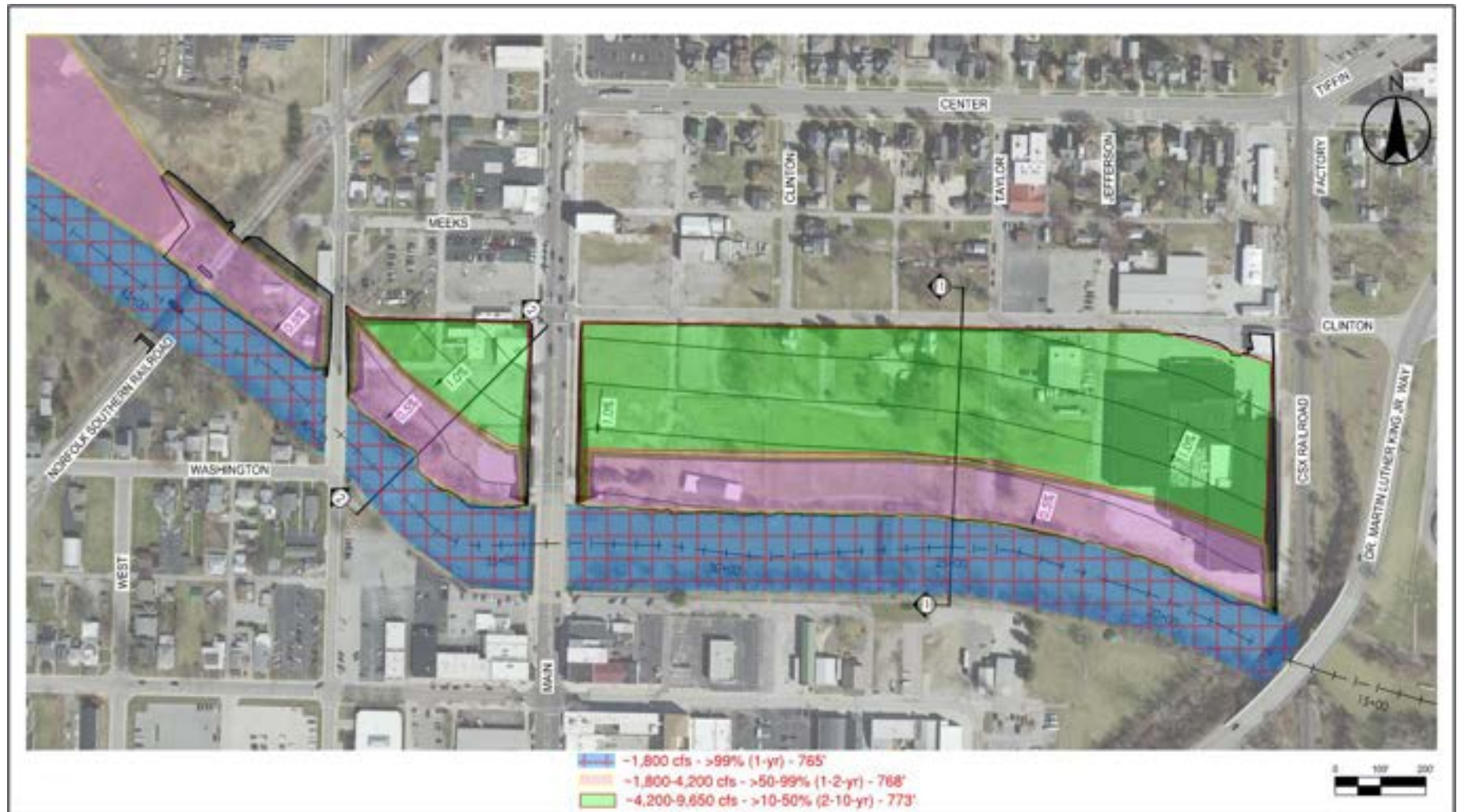
Figure 19 – Plan View of Concept 1 Anticipated Flood Extents and the associated Blanchard River Discharge / Recurrence Interval
