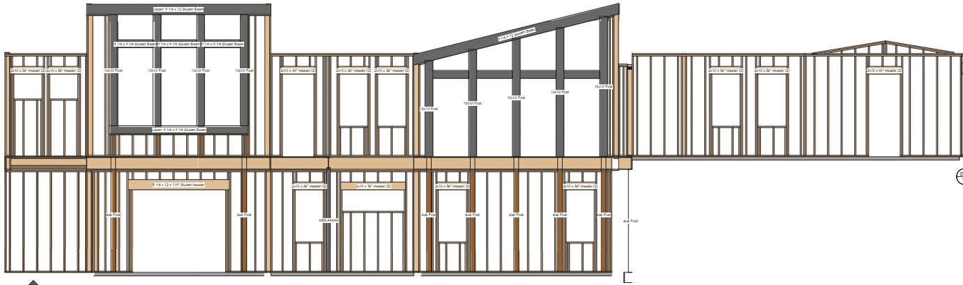
F2 REAR WALL FRAME DETAIL 1/4"=1'
