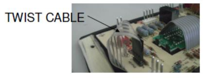
STEP 7. PLUG IN YOUR NEW KEYPAD TO THE KEYPAD CONNECTOR. <u>MAKE SURE YOU HAVE A</u> <u>TWIST THE CABLE</u>. THIS IS DIFFERENT FROM THE HAYWARD KEYPAD. I CHANGED THE CIRCUITRY SO AS NOT TO COPY HAYWARD'S DESIGN! IF YOU PLUG IT IN WRONG YOUR KEYPAD WILL NOT WORK PROPERLY.
