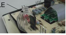
STEP 7. PLUG IN YOUR NEW KEYPAD TO THE KEYPAD CONNECTOR. <u>MAKE SURE YOU HAVE A</u> <u>TWIST THE CABLE</u>. THIS IS DIFFERENT FROM THE HAYWARD KEYPAD. I CHANGED THE CIRCUITRY SO AS NOT TO COPY HAYWARD'S DESIGN! IF YOU PLUG IT IN WRONG YOUR KEYPAD WILL NOT WORK PROPERLY.
