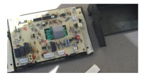
STEP 4. YOU SHOULD NOW BE ABLE TO SEE THE KEYPAD CONNECTION. UNPLUG IT AND THEN IF YOU CAN REMOVE THE OLD KEYPAD FROM THE FRONT PLASTIC. YOU MAY HAVE TO LOOSEN THE SCREWS ON THE PRINTED CIRCUIT BOARD TO REMOVE THE CONNECTOR TAIL.
